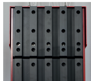
Rifle sights Alignment is performed by looking through the aperture in the right side of the heat sink.
